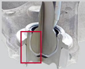
BALL JOINT Sealed plastic bearing design
