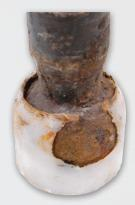
**OE-STYLE PLASTIC BEARING** Excessive heat and non-greasable sealed design can lead to premature failure
