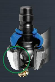
Innovative threaded ball joint design enables engineered greaseable self-lubricating sintered metal to be placed in unitized aluminum control arms.
