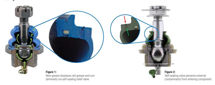
Mevotech Supreme and TTX steering and suspension components are pre-greased from the factory. However, it is suggested to introduce one or two pumps of grease during installation. After installation, it is recommended to inspect and re-grease at every vehicle oil service interval.
